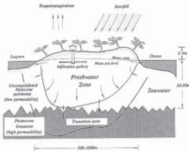
**Figure 4: Cross section through a small coral island showing main features of a freshwater lens (exaggerated vertical scale) and location of an infiltration gallery.**
