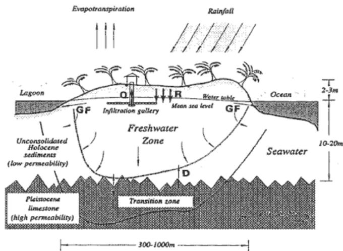
Figure 1: Typical cross section through a coral island with a freshwater lens
