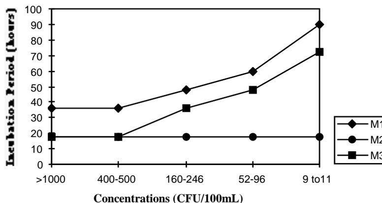
Fig. 1. Incubation period for the three media at different concentrations of faecal coliforms at 37°C
