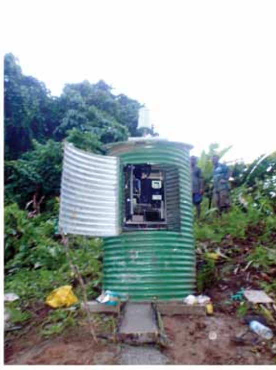
Lape River, typical bubbler system installation including raingauge and solar panels on roof
