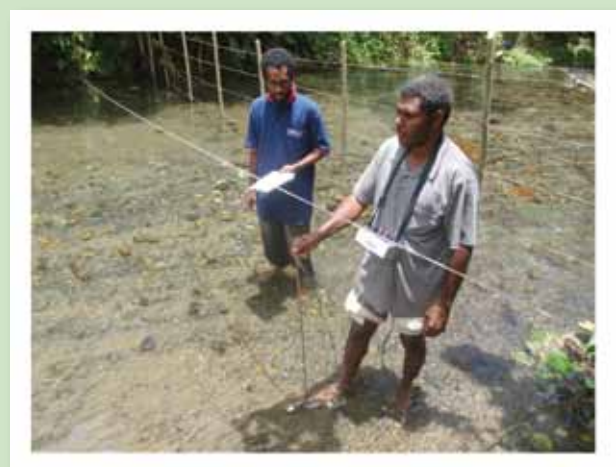
Undertaking low flow discharge measurement, La Colle River
