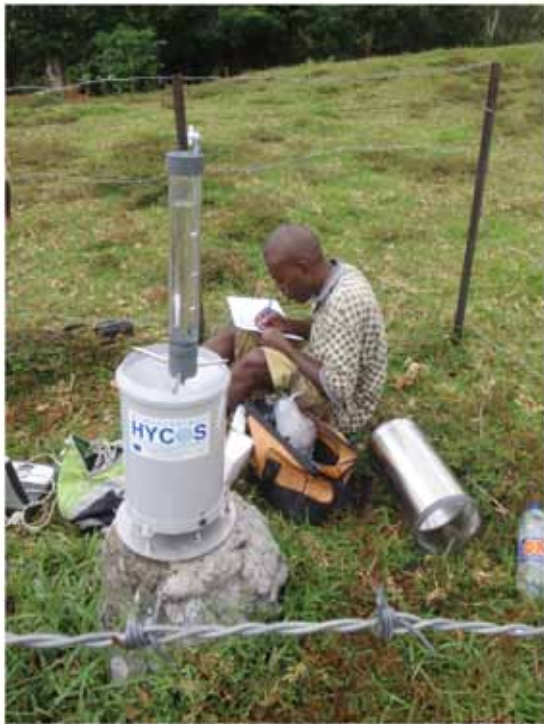
Epule raingauge, calibration check following installation
